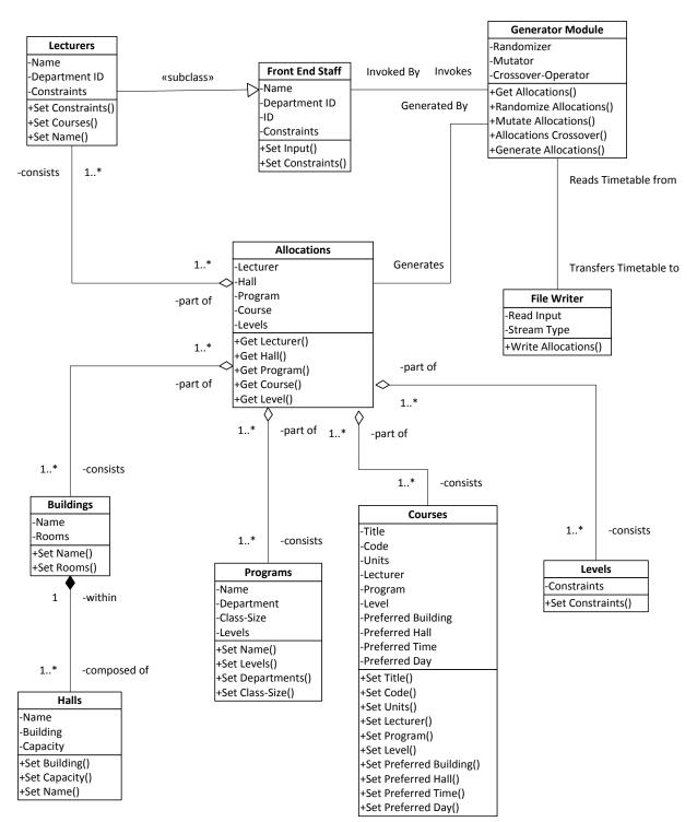
Figure 2.: Class Diagram to show the relationships between the different classes associated with the system
